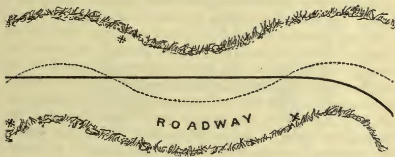
FIG. 49.—Diagram illustrating a straight course avoiding sharp turns and side-slips at points marked by crosses (X X X). Dotted line, course to avoid; straight line, best course to follow.
